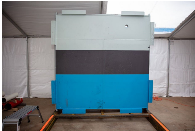
Figure 1: Dry hull test panel (1) . Large circular defects representing general corrosion and small blind holes representing pitting corrosion were machined into the back side of the plate at depths ranging from 10 to 50% of the material thickness, and covered with insulation so they were not visible to the Innovators.
