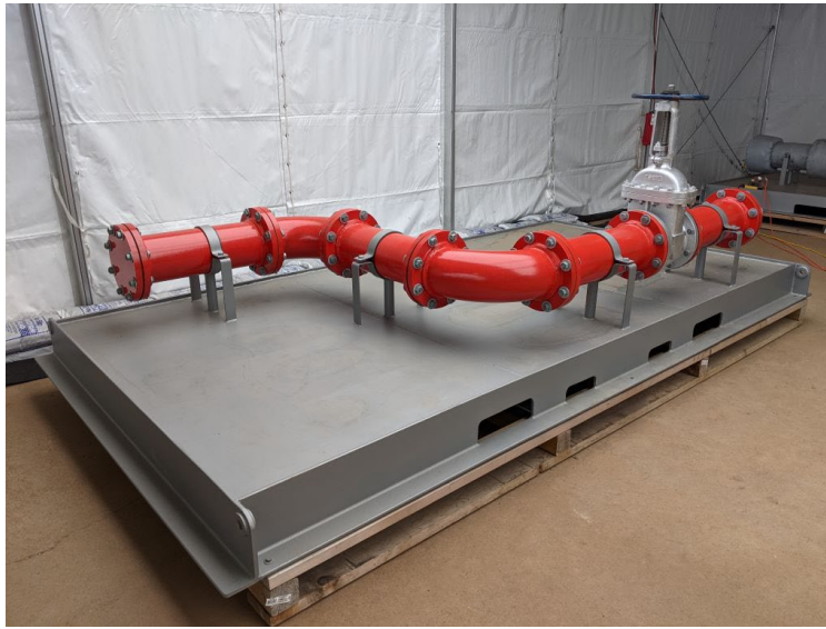
Figure 5: Steel fuel oil transport pipe test panel. Large circular defects representing general corrosion and small blind holes representing pitting corrosion were machined into the inner surfaces of the pipe at depths ranging from 10 to 50% of the pipe wall thickness.
