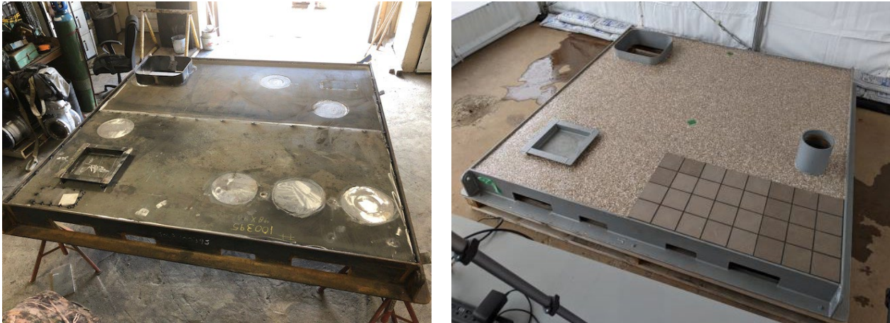
Figure 3: Seamless decking test panel before (left) and after (right) coating. Large circular defects representing general corrosion and small blind holes representing pitting corrosion were machined into the front side of the plate at depths ranging from 10 to 70% of the material thickness, and covered by seamless decking or quarry tile.
